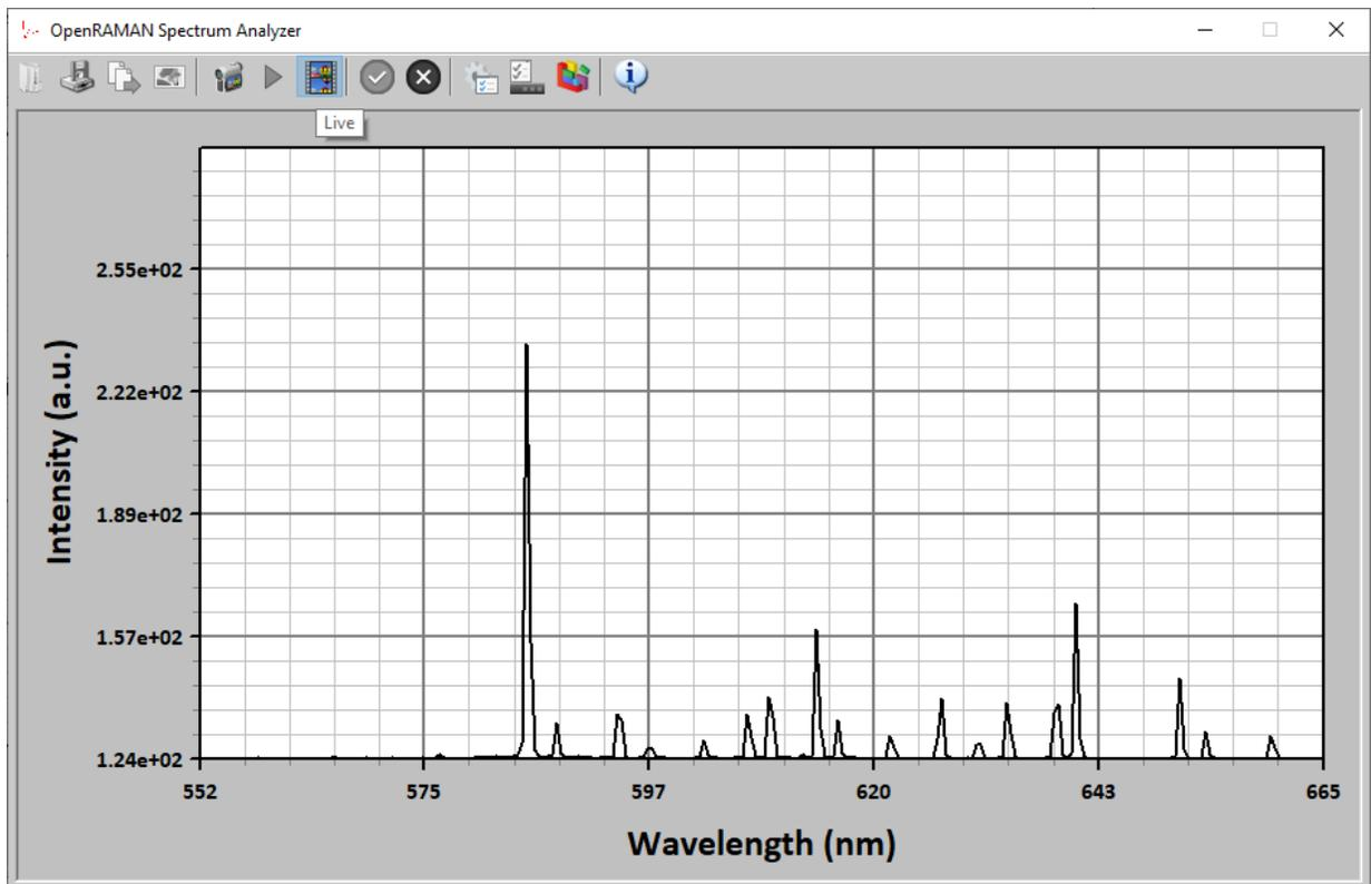
Live capture will usually be necessary when aligning the spectrometer. Some of the functionalities are disabled in the live capture mode.
