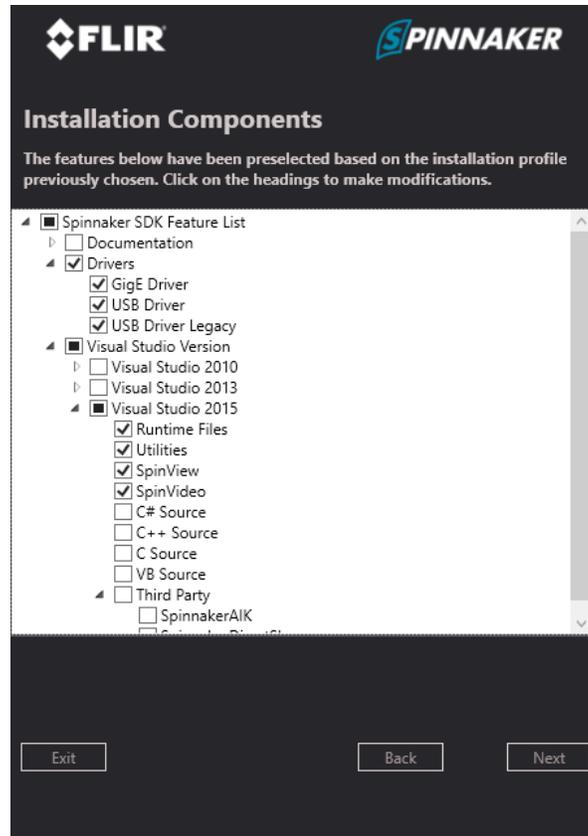
When using GiGe camera, run the configuration tool to set up your Ethernet adapter to work with cameras and connect to the camera using the SpinView program to set up a correct IP address. This should be done only once when you setup your system to work with the spectrometer.
