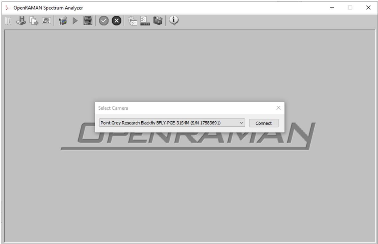
Spectrum Analyzer is compatible with both the Starter and Performance Editions but also support any spectrometer for which a .dll library has been included to connect to. By default, the application will load almost any recent PtGrey monochrome cameras. So far, the program has been validated with the following camera models:
