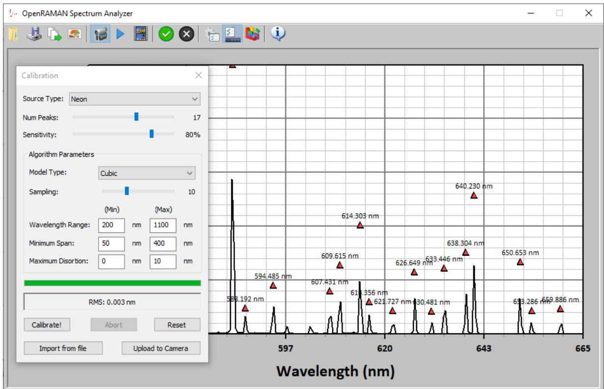
The algorithm that was developed to calibrate the system is relatively robust but may need some tweaking. You can either choose from a Linear model or from a Cubic model. Cubic model offers more flexibility but is slower to fit. If the algorithm does not fit properly, you can try increasing the sampling parameter. Increased sampling will run slower.
