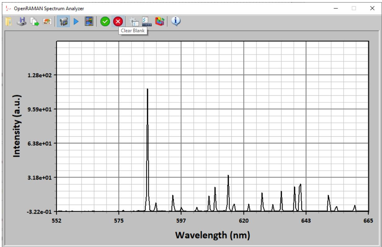
Blank data will be saved in the Spectre file next to the data so that you can eventually disable it later. Blank data will not be saved separately to CSV files and CSV or clipboard data will always have the blank subtraction enabled.
