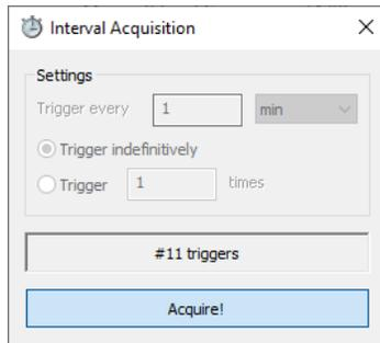
To perform time-lapse acquisitions, start the Spectrum Analyzer program and connect to the spectrometer. Adjust the exposure and gain for your experiment and enable the automatic logging of spectra. Eventually take a blank measurement if you wish to.
