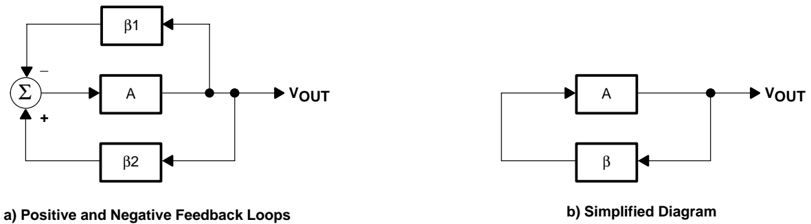
Figure 5. Block Diagram of an Oscillator
